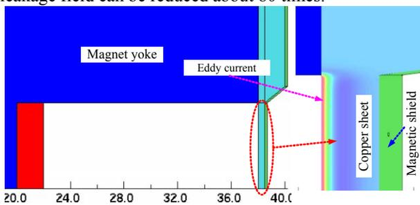
Figure 4: Septum magnet with magnetic shield
