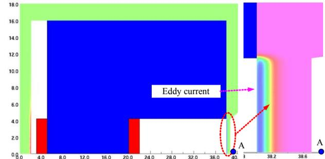
Figure 1: Cross section of septum and eddy current distribution
