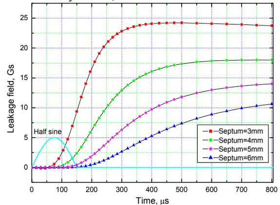
Figure 2: Leakage field varies with time (point A)
