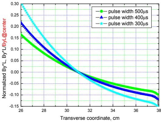
Figure.8: Integrated gap field uniformity degradation
