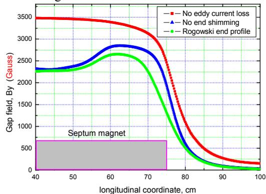
Figure 7: Longitudinal field distribution at magnet end
