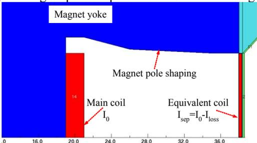
Figure 10: Magnet pole shaping
