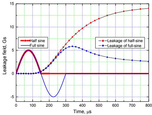
Figure 3: Leakage field with different excitation (Septum thickness is 5 mm)
