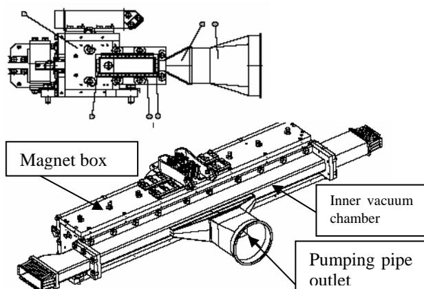
Figure 3: Cross-section of the Storage Ring septum magnet
