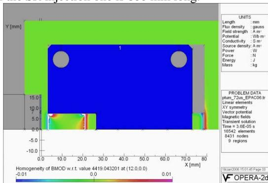
Figure 1: Field homogeneity and current calculations
