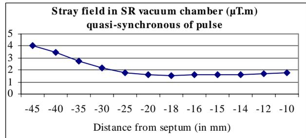
Figure 5: Strongly reduced stray field in final status
