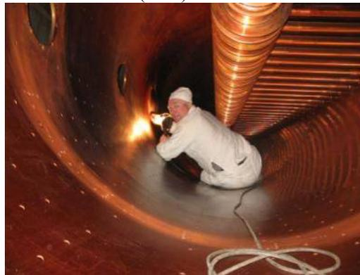
Figure 1: Inner view of LU-20 resonator.
